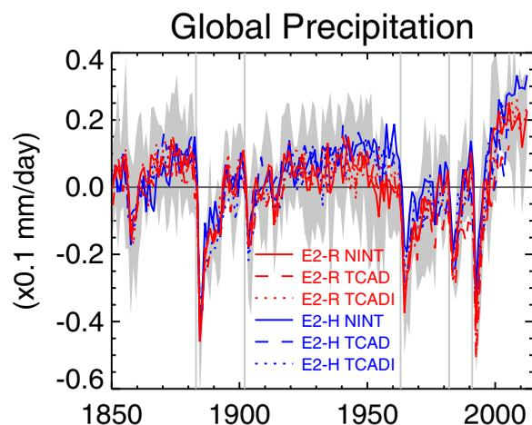
**Figure 21.** Global precipitation anomaly (in tenths of a  $\text{mm day}^{-1}$ ). Shading represents variations among ensemble members within the E2-R NINT ensemble (plus or minus two standard deviations). Major volcanic eruptions are marked with vertical lines.
