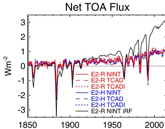
**Figure 18.** Net radiative flux at TOA ( $\text{Wm}^{-2}$ ) for the ensemble averages. The black line shows instantaneous radiative forcing at the tropopause (“iRF”) for the E2-R NINT ensemble. Ensemble values are global and annual averages.
