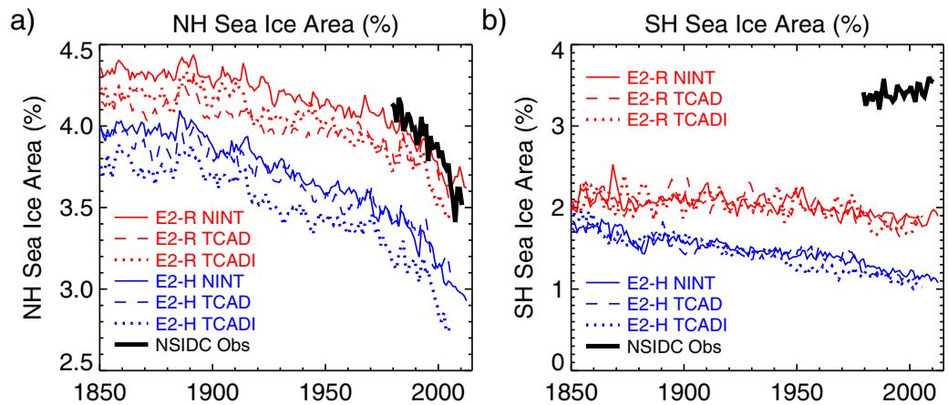
**Figure 16.** Model sea-ice area compared to passive microwave retrievals from the National Snow & Ice Data Center for the (a) Northern Hemisphere and (b) Southern Hemisphere. Plotted area is an annual average and hemispheric sum expressed as a percentage of the total hemispheric area.
