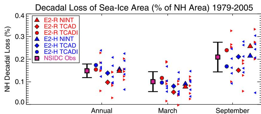
**Figure 17.** Change in NH sea-ice area (per decade and as a percentage of total hemispheric area) between 1979 and 2005. The observed value from the NSIDC is in purple with its uncertainty in black (corresponding to two standard deviations of interannual variability). Ensemble average change is shown as triangles (NINT), diamonds (TCAD), and circles (TCADI), with change for individual ensemble members plotted as small triangles.
